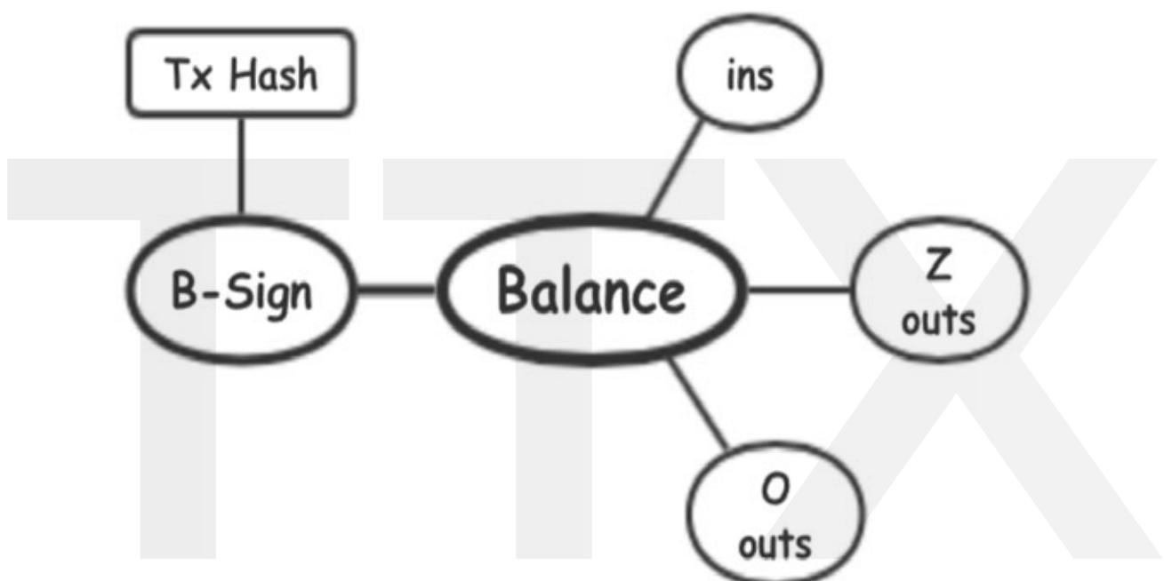
Tx pack ins, Z outs, and O outs together, how to prevent malicious attackers from tampering with the data inside and secure the assets, we do so by introducing perdesen commitment, whose homomorphic encryption property allows the verifier to confirm that Balance must be balanced, i.e., input equals output, without knowing the details of the message.
