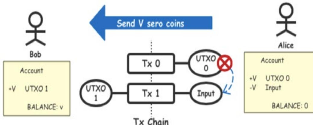
As shown above, there are two types of records in the UTXO mode, Input and Output for the transaction initiator, and this Output is the Unspent Output (UTXO) in the view of the transaction receiver until the transaction receiver initiates another transaction and specifies an Input to nullify this UTXO. The records in the transaction are always linking the various Inputs and Outputs. In this model, ACCOUNT is not required as a state summary.
